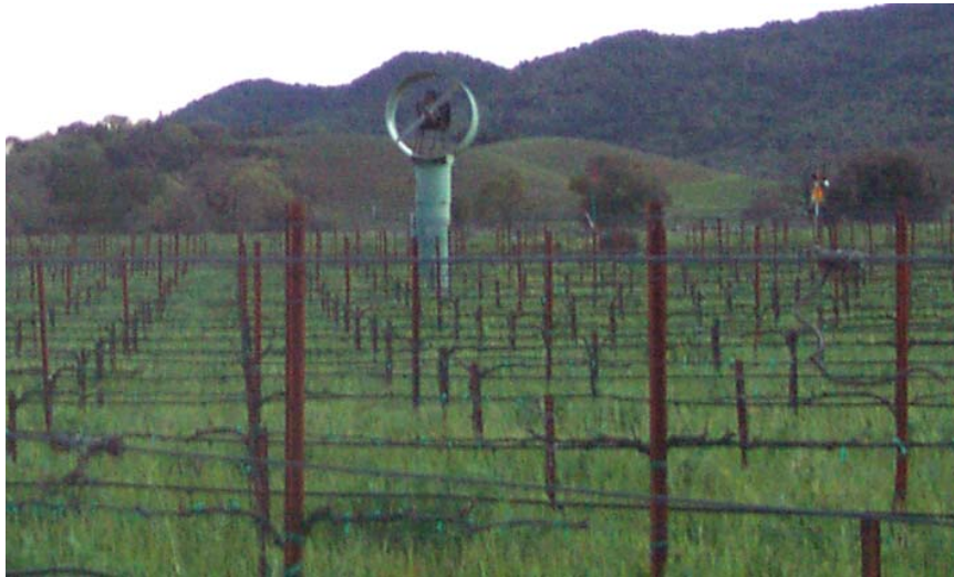
One type of wind machine used to reduce frost damage in vineyards.
