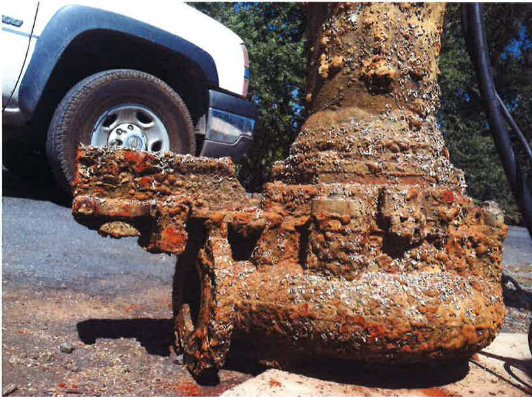
Photo 2 - Failed PumpEx Submersible pulled from wet pit
