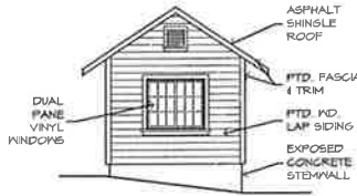
SHED EAST ELEVATION SCALE: 1/8" = 1'-0"
