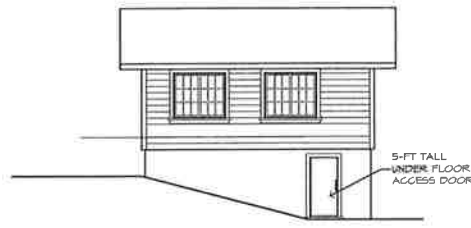
SHED NORTH ELEVATION SCALE: 1/8" = 1'-0"
