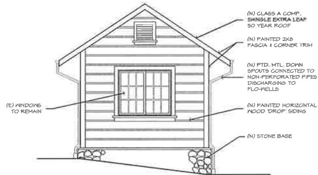
SHED EAST ELEVATION
