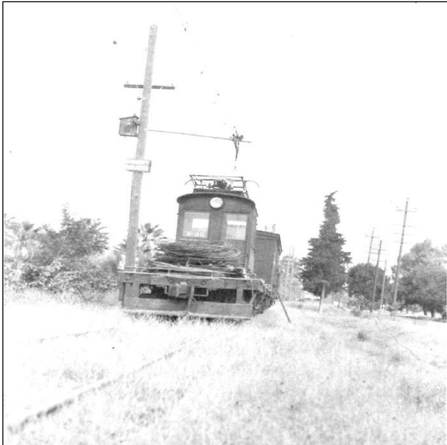
Figure 10: Electric locomotive #98, the first electric car to operate on the railway that is shown here taking up the rails near Rutherford after the abandonment of passenger service in 1937 (Swett and Aitken 1975: 401).
