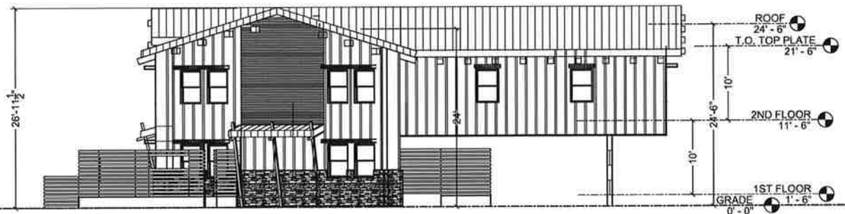
4 SOUTH (WASHINGTON STREET - SIDE) ELEVATION 1/8" = 1'-0"
