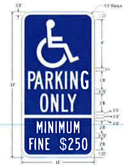
R99B (CA) COLORS: BORDER & LEGEND - WHITE (RETROREFLECTIVE) BACKGROUND - BLUE (RETROREFLECTIVE)
