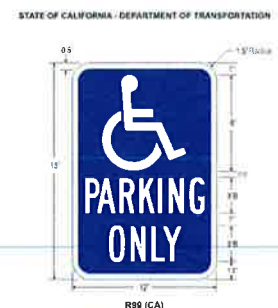
R99 (CA) COLORS: BORDER & LEGEND - WHITE (RETROREFLECTIVE) BACKGROUND - BLUE (RETROREFLECTIVE)
