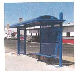
17' SIERRA DOME ROOF SHELTER WITH BRONZE LEXAN ROOF PANELS, PERFORATED METAL PANELS AT THE REAR AND DOWNSTREAM END WALL, DECORATIVE SAHUARO POST UPSTREAM, DUSK TO DAWN SOLAR ILLUMINATION--- BENCH BY OTHERS
