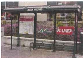
13' SIERRA DOME ROOF TRANSIT SHELTER WITH BRONZE LEXAN ROOF PANELS, ROOF ENDS CLOSED OFF WITH ALUMINUM, TWIN DECORATIVE REAR POSTS, 3/8" CLEAR TEMPERED SAFETY GLASS WALLS, INTEGRATED REAR WALL MAP CASE, WIRE GRID BENCH WITH ANTI-VAGRANT BARS, AGENCY BRANDING
