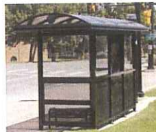
18' DOME ROOF TRANSIT SHELTER WITH BRONZE LEXAN ROOF PANELS, FRAMED PERFORATED ALUMINUM ROOF PANELS AT THE BOTTOM AND 3/8" GLASS AT THE TOP OF THE REAR AND END WALLS, INTEGRATED REAR WALL MAP CASE, PERFORATED METAL BENCHES, INTEGRATED BIKE LOOPS AT EACH END-END VIEW
