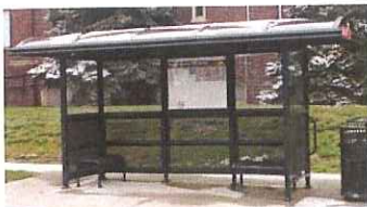
18' DOME ROOF TRANSIT SHELTER WITH BRONZE LEXAN ROOF PANELS, FRAMED PERFORATED ALUMINUM ROOF PANELS AT THE BOTTOM AND 3/8" GLASS AT THE TOP OF THE REAR AND END WALLS, INTEGRATED REAR WALL MAP CASE, PERFORATED METAL BENCHES, INTEGRATED BIKE LOOPS AT EACH END-FRONT VIEW
