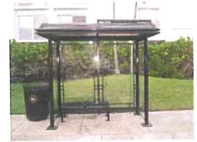
9' SIERRA DOME ROOF TRANSIT SHELTER WITH BRONZE LEXAN ROOF PANELS, 3/8" VICTORIAN STYLE FRITTED GLASS PANELS AT THE REAR AND END WALLS, PERFORATED METAL BENCH WITH ONE ANTI-VAGRANT BAR-SOLAR ILLUMINATION
