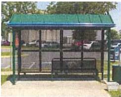
13' SIERRA HIGH PEAK ROOF TRANSIT SHELTER SHELTER WITH ALUMINUM ROOF PANELS, DECORATIVE BATTENS, PERFORATED METAL REAR WALL WITH ACRYLIC INSERTS, 3/8" GLASS END WALLS, INTEGRATED END WALL MAP CASE, PERFORATED METAL BENCH WITH BACK AND PERFORATED METAL TRASH RECEPTACLE
