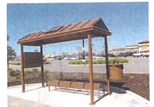
13' SIERRA HIGH PEAK ROOF TRANSIT SHELTER WITH ALUMINUM ROOF PANELS, DECORATIVE BATTENS, 3/8" GLASS REAR AND END WALLS, INTEGRATED END WALL MAP CASE, PERFORATED METAL BENCH WITH ANTI-VAGRANT BARS - SOLAR ILLUMINATION
